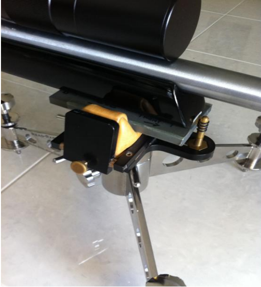
Front Rest showing side tensioning screws
